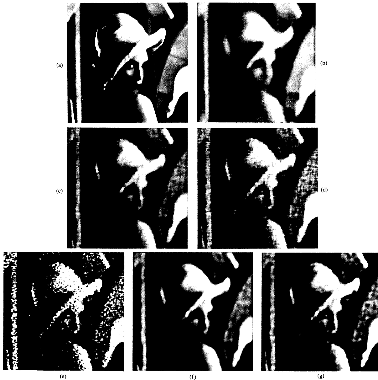
Fig. 4. (a) Original Lena 128 by 128 image; (b) Distorted image; SNR = 20 dB and 7 by 7 blur. Restored images by (5): (c) Q = I, \lambda_{CLS} . (d) Q = I, \lambda_{CV} . (e) Q = I, \lambda_{ML} . (f) Q = Q_{2DL}, \lambda_{CLS} .
