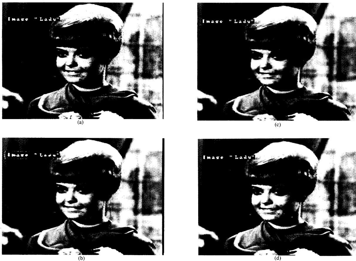
Fig. 7. Reconstructed images of "Karen with Text" using (b) adaptive DCT method [3], (c), and (d) prioritized DCT method. (a) Original image. (b) 1.00 b/pixel (ADCT). (c) 0.50 b/pixel (PDCT). (d) 1.00 b/pixel (PDCT).
