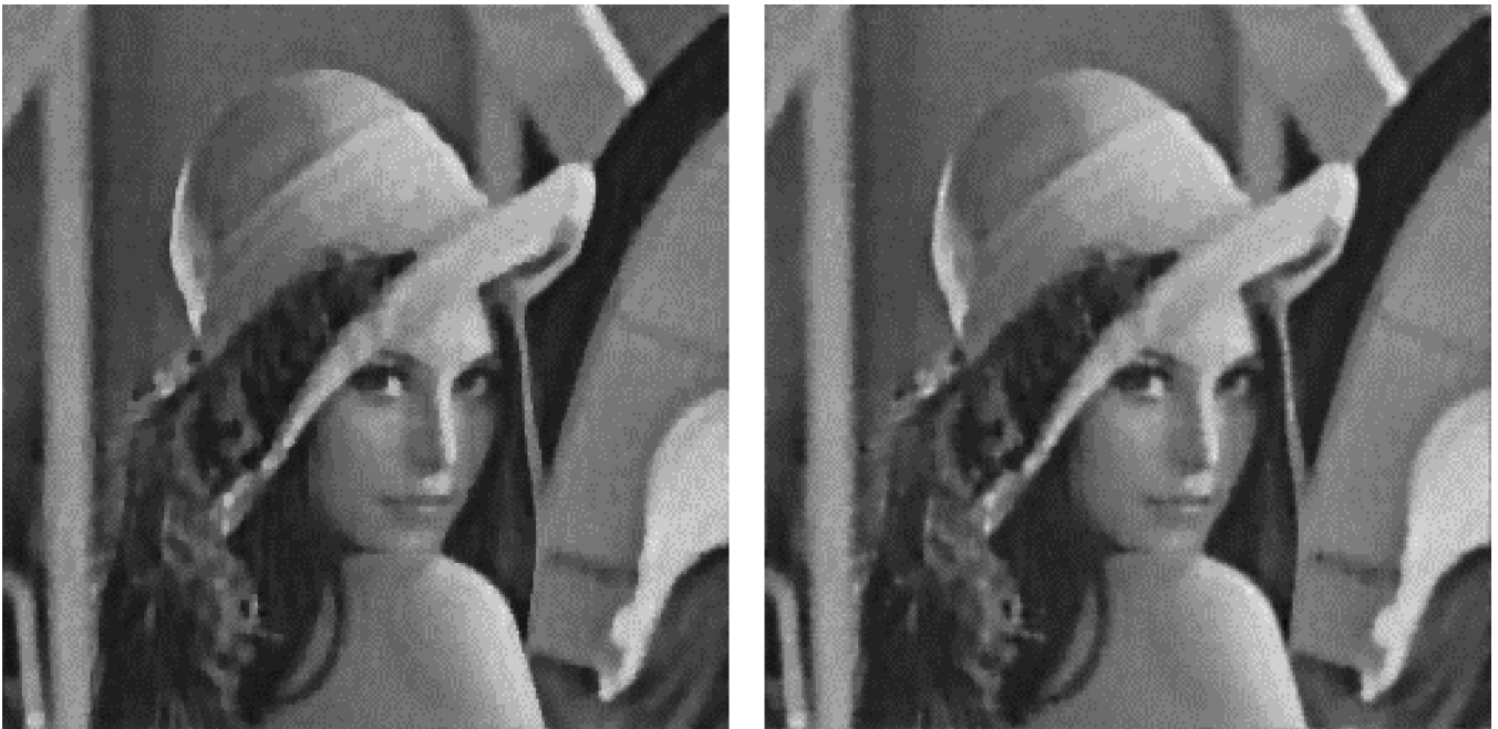
Fig. 1. (Continued.) (i) MAP non Stationary restoration, ISNR = 5.63 dB, l = 2.2 . (j) Bayesian non stationary restoration, ISNR = 5.22 dB, l = 2.2 .
