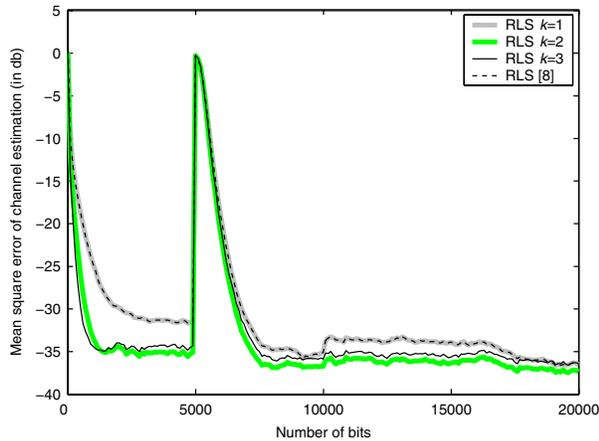
Fig. 1. Performance of the proposed RLS channel estimation schemes versus the method of [8]; noise power 20 db.
