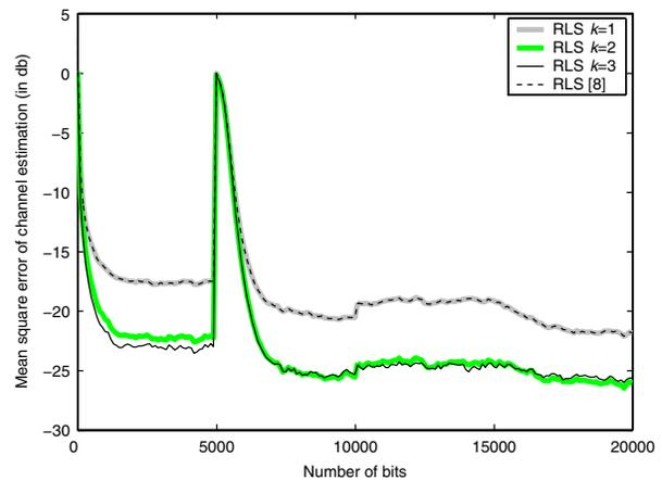
Fig. 3. Performance of the proposed RLS channel estimation schemes versus the method of [8]; noise power 10 db.
