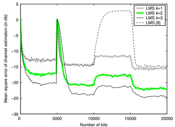
Fig. 4. Performance of the proposed LMS channel estimation schemes versus the method of [8]; noise power 10 db.
