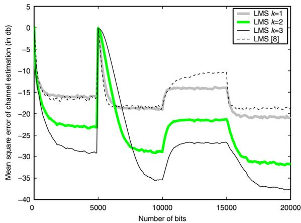
Fig. 2. Performance of the proposed LMS channel estimation schemes versus the method of [8]; noise power 20 db.
