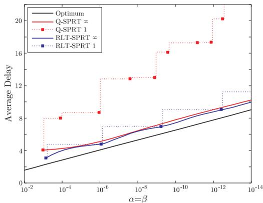
Fig. 4. Average detection delay vs error probabilities  $(\alpha, \beta)$  for optimum centralized, Q-SPRT and RLT-SPRT with 1,  $\infty$  number of bits.
