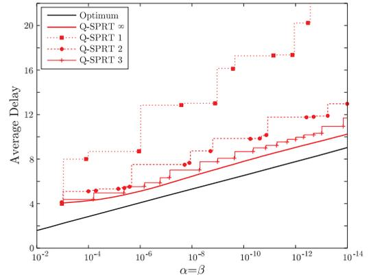
Fig. 2. Average detection delay vs error probabilities  $(\alpha, \beta)$  for optimum centralized and Q-SPRT with 1, 2, 3,  $\infty$  number of bits.
