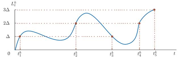
Fig. 1. A realization of a local LLR process and its sampling times when level-triggered sampling with sampling level  $\Delta$  is applied.
