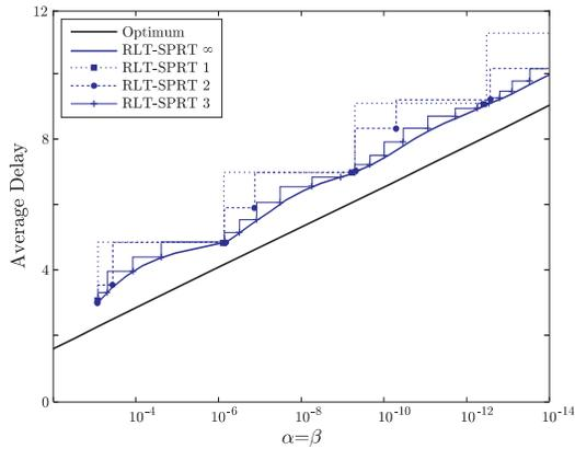
Fig. 3. Average detection delay vs error probabilities  $(\alpha, \beta)$  for optimum centralized and RLT-SPRT with 1, 2, 3,  $\infty$  number of bits.
