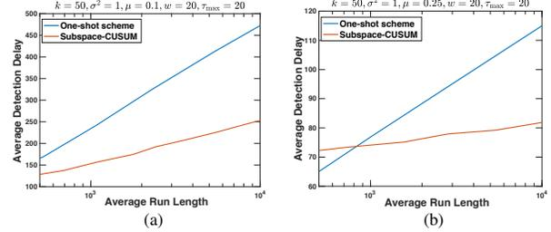
Fig. 2. Comparison of Average detection delay as a function of Average run length for Subspace-CUSUM and One-shot detection scheme.
