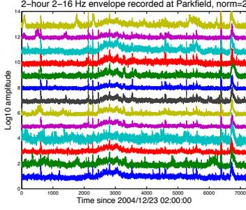
Fig. 3. Raw data from 13 sensors.
