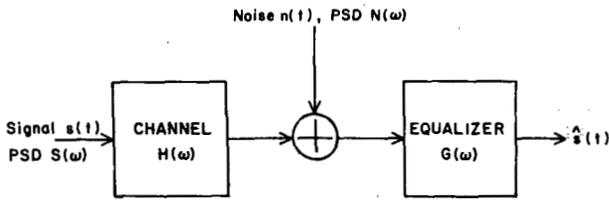
Fig. 1. Equalization of noisy linear channel.
