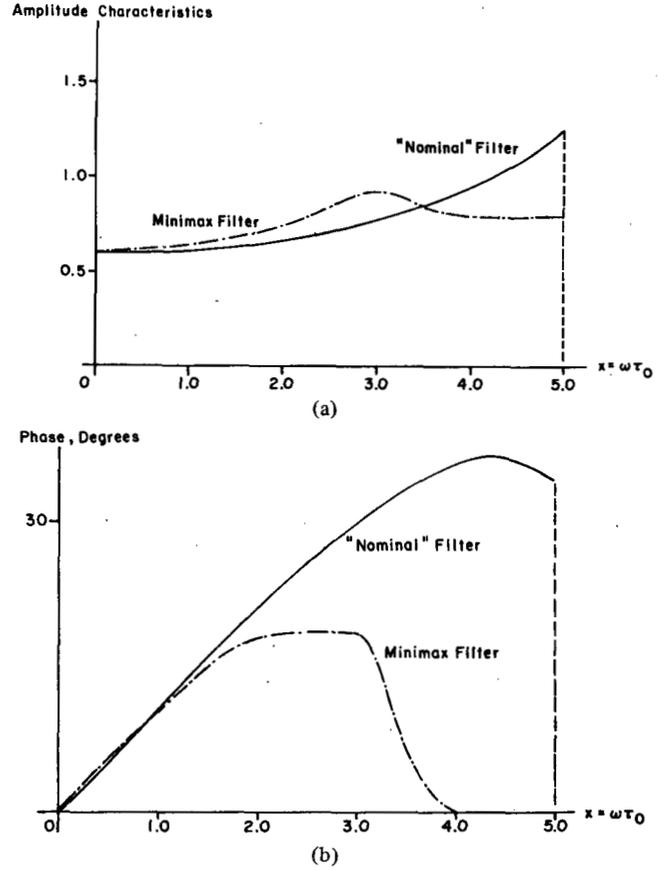
Fig. 5. (a) Amplitude characteristics of nominal and minimax filters ( $a_0 = 0.6$ ,  $x_0 = \omega_0\tau_0 = 5$ ,  $N_0/S_0 = 0.1$ ). (b) Phase characteristics of nominal and minimax filters ( $a_0 = 0.6$ ,  $x_0 = \omega_0\tau_0 = 5$ ,  $N_0/S_0 = 0.1$ ).
