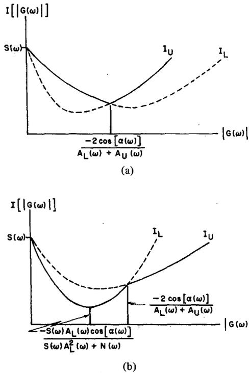
Fig. 3. Minimization of  $I(|G(\omega)|)$  for solution of minimax filter amplitude [see (13)].
