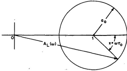
Fig. 4. Geometry for computing amplitude and phase bounds for multipath channel example.
