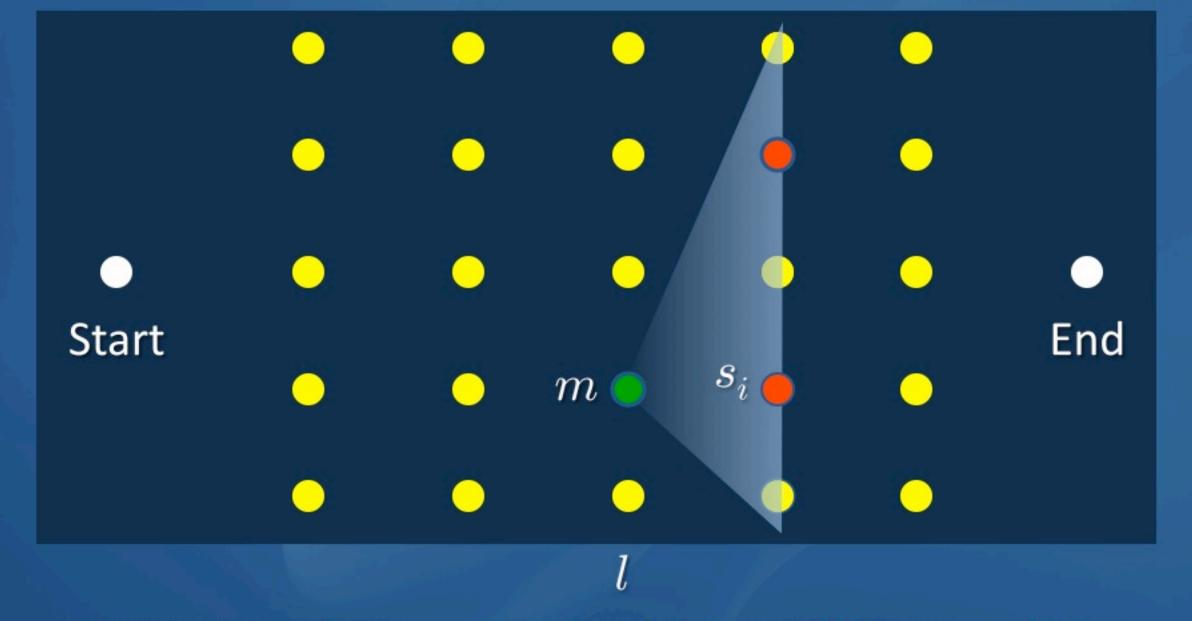
Vehicle is at node m of column l and observes state  $s_i$  of column  $l\!+\!1$
